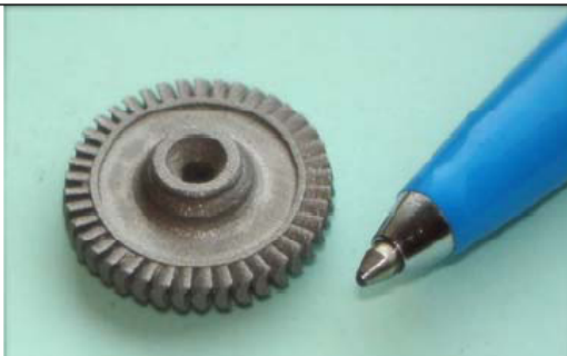
Figure 7 Fully dens cogwheel in SS, 35µ resolution xyz, Ink Jet Man. (copyright Fcubic)
