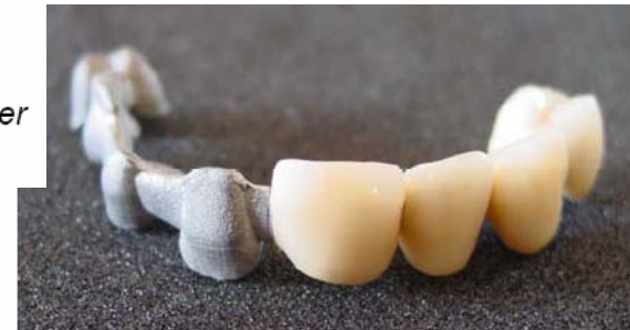
Figure 6 Tooth prostheses in CoCr alloy, solid phase laser sintering (copyright Phenix)
